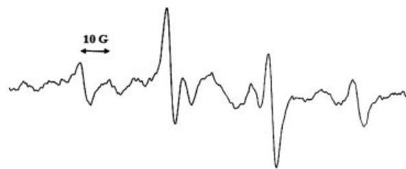
Figure 5 ESR spectrum observed in the bulk polymerization of DMVP with DCPO at 110°C ( [\text{DCPO}] = 5.0 \times 10^{-2} mol/L).
